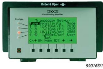
NEXUS units with embedded software version 2.0 or later can identify transducers with built-in TEDS that comply with the IEEE 1451.4 standard. Such transducers can be identified by their type numbers and their sensitivities read into the NEXUS unit.
